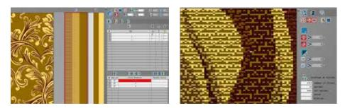
Jacquard Processing defines and compiles the complete working process from designs edited in Scope all the way to the control information for the Jacquard weaving machine.
