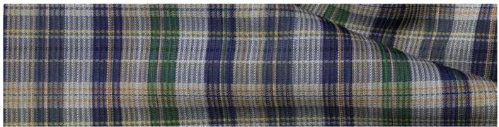
Based on a Jacquard or Dobby weaving file the 3D Fabric Simulation mirrors the entire complex process of weaving and gives you a realistic impression of your fabrics. It does not matter if you want to use the simulation for the presentation to your clients or just for checking the weaving file for yourself. The result will help you in any case.
